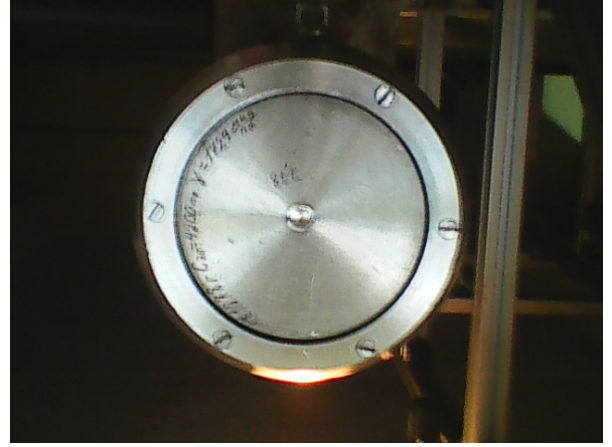
Fig. 4. Piezoelectric circular piston with diameter of the diaphragm 98 mm.
